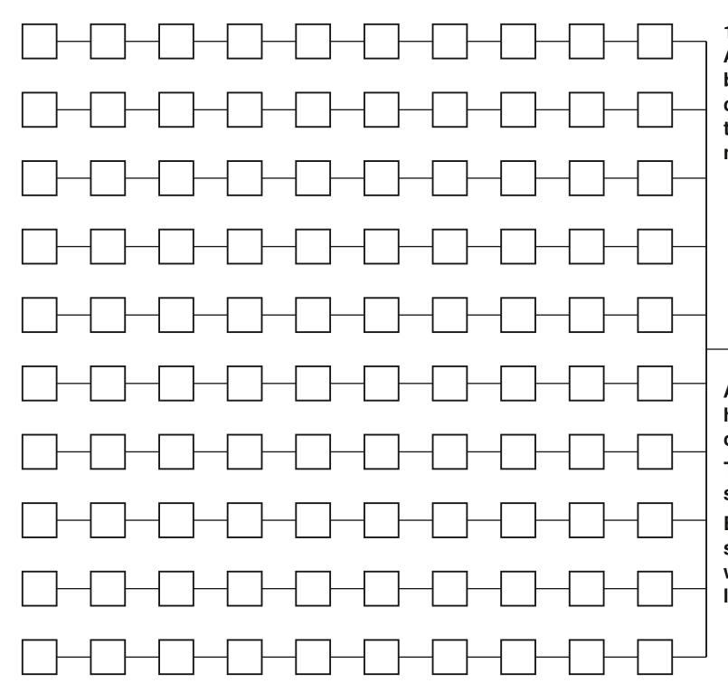
100 houses, each has a 25 A three-phase connection, but all together are connected to a 400 kVA transformer on the medium-voltage network.
